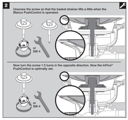
2. Adjusting the sealing plug screw System check:
