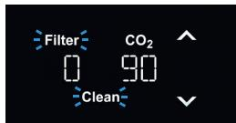
When the filter has run out or it is time for cleaning, the 'Clean' and 'Filter' symbols will flash. The system needs to be cleaned and a new filter installed.
