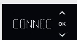
After pressing 'OK', the appliance displays the message 'CON OFF'. Use the arrow keys to change to 'CON ON', 'CON RES' or 'BACK', and confirm by pressing 'OK'. Return to the menu by selecting 'BACK' and confirm by pressing 'OK'.
