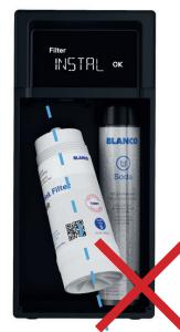
Screw in the filter with roughly two twists. When inserting the new filter, make sure that it is put in straight, not slanted! You can tilt the filter forward in the appliance in order to screw it in and out.
