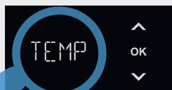
After confirming with 'OK', the set target temperature in the cooling and carbonation unit is displayed and can be set between 4 and 10 °C using the arrow buttons. Please note: the appliance takes a little time to reach the set temperature.
