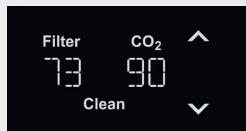
Normal operating mode with remaining capacity for filter and CO<sub>2</sub> displayed (in %). The left-hand figure shows the remaining capacity of the filter. The right-hand figure shows the remaining capacity of the CO<sub>2</sub> cylinder.
