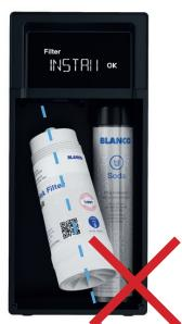
Screw in the filter with roughly two twists. When inserting the new filter, make sure that it is put in straight, not slanted! You can tilt the filter forward in the appliance in order to screw it in and out.
