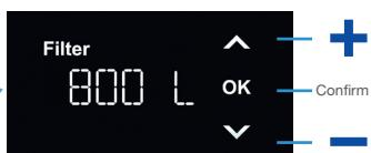
Read off the filter capacity from the filter documents. Enter the figure manually. Confirm by pressing "OK".
