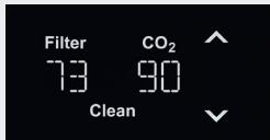
Normal operating mode with remaining capacity for CO<sub>2</sub> and filter displayed (in %). The left-hand figure shows the remaining capacity of the filter. The right-hand figure shows the remaining capacity of the CO<sub>2</sub> cylinder.
