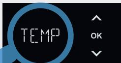
After confirming with 'OK', the set target temperature in the cooling and carbonation unit is displayed and can be set between 4°C\* and 10°C using the arrow buttons. Please note: the appliance takes a little time to reach the set temperature.
